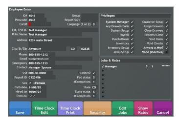
Under the Security button; edit the user security fields. RPOWER will use the Email or SMS and Emergency fields for password recovery. Password recovery is only permitted with successful confirmation of matching PIN#1 and PIN#2 set for this user profile.
